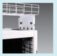
Specially designed brackets mount to the top of LX cabinets and support Cablofil® cable tray, providing a cost-efficient and more compact alternative to ceiling suspended cable management. FAS style tabs secure tray without the need for additional hardware or tools.
